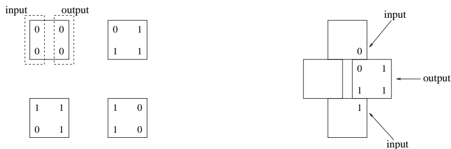
Figure 1: The set of four tiles on the left implements the operation \oplus . A tile glues to other tiles only if their corner labels match. On the right operation 0 \oplus 1 = 1 is performed. The input tiles are preassembled and the correct output tile simply attaches itself to the pattern, effectively obtaining the value of the output bit.
